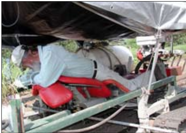
The water jets and Drängen controls are operated by foot pedals.
