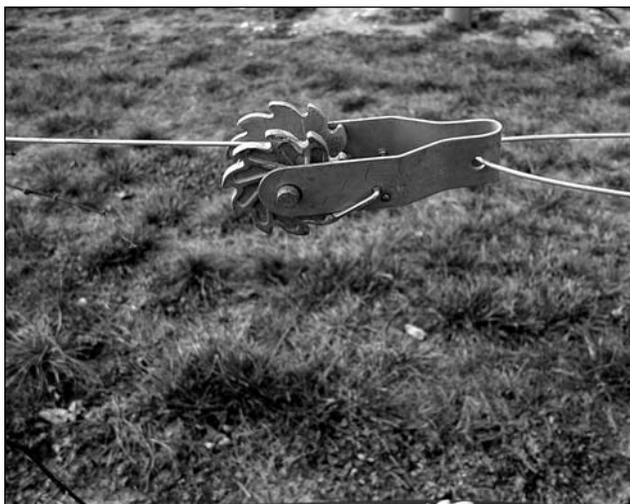
**Fig. 6-9.** In line strainers
