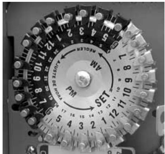
The 24-hour timer to control day/night cycle
