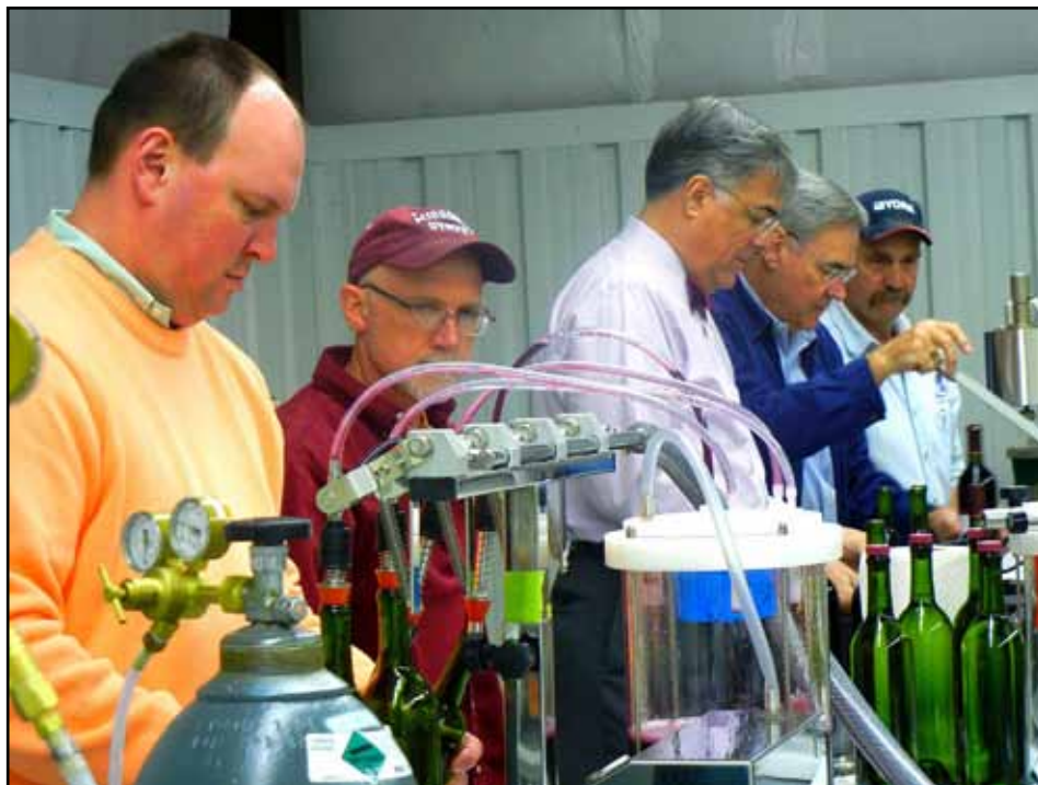
Darin Link (far left) sparges and fills the bottles of wine, checks the level of wine in the bottle, and uses the corking machine (not shown) to stopper the bottles. Dr. James Cofer (middle) applies the front and back Missouri State wine labels and Dr. Anson Elliott (middle right) puts the capsule on the bottle and heats it to seal while Dr. Karl Wilker (middle left) and C. J. Odneal (far right) supervise the bottling line.
