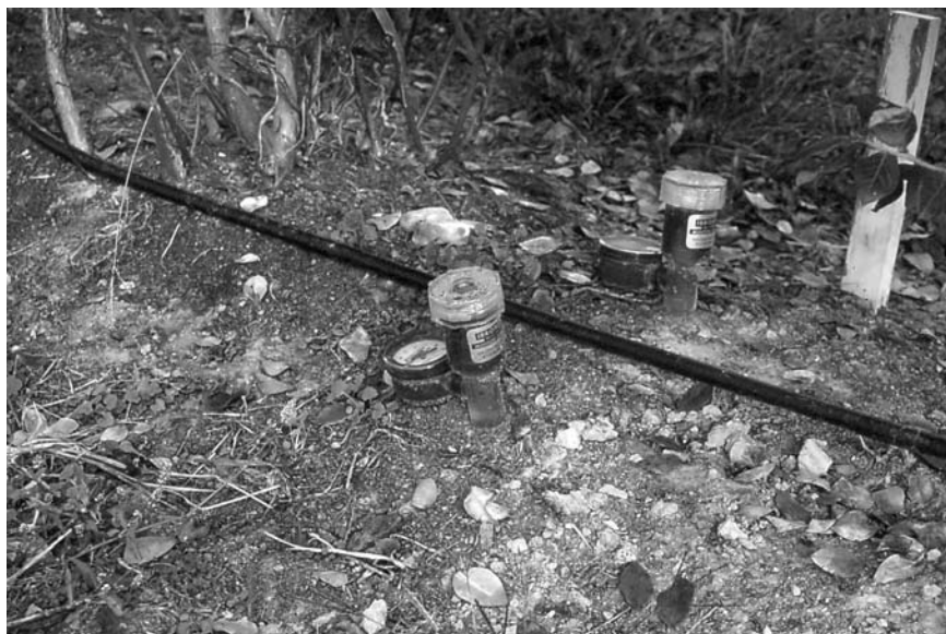
Fig. 4. Tensiometers placed near trickle irrigation line.
